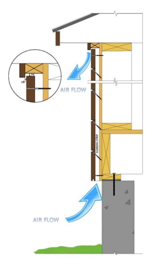
Due row of vertical furring strips must be applied to the sheathing followed by a horizontal row before cladding can be installed to provide air flow behind cladding.
