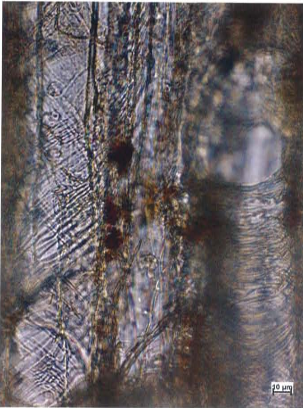
Figure 1: specimen B31; beech, caverns of soft rot fungi, M 600:1
