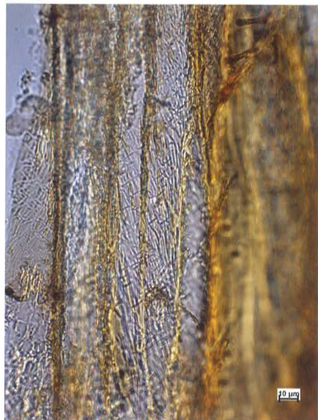
Figure 2: specimen 1; TMT Yellow Poplar, caverns of soft rot fungi, M 600:1
